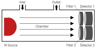
Besides NDIR type sensor, AM319 uses a photoacoustic CO<sub>2</sub> sensor to measure the CO<sub>2</sub> level by measuring the sound via a MEMS microphone.
