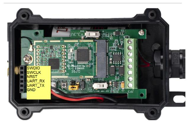
In the PC, you need to set the serial baud rate to **9600** to access the serial console for LDDS20. LDDS20 will output system info once power on as below:
