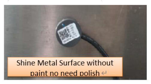
Step3: Test the installation point.
