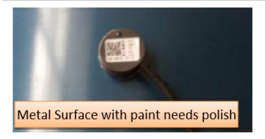
No polish needed if the container is shine metal surface without paint or non-metal container.
